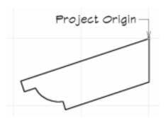
3. "Slabify" your profile using ArchiCAD's "transform" capabilities as follows: double-click on the Slab tool and set the thickness of the slab to be the thickness of your rafter, let's say 3 1/2 inches, and the elevation "to project Zero" to "0." Specify all other settings like model attributes, line color, section attributes, and layer. Press OK.
